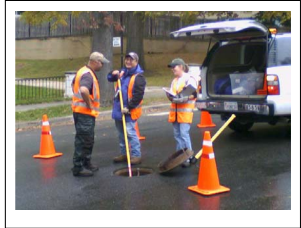
Stormwater Grab Sampling.
