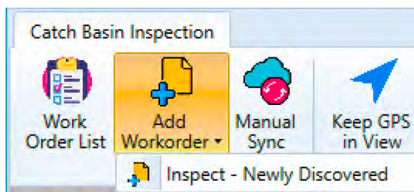
Figure 49 - Add Workorder dropdown menu for INSP mode of operation of CB App
