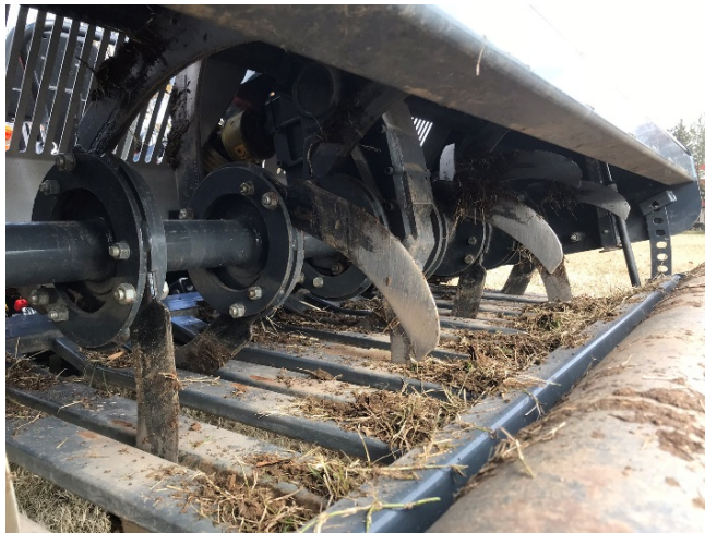
Photo 1 (left): Rotary shaft and blades of rotary de-compactor and Photo 2 (right): tracks left after rotary de-compaction
