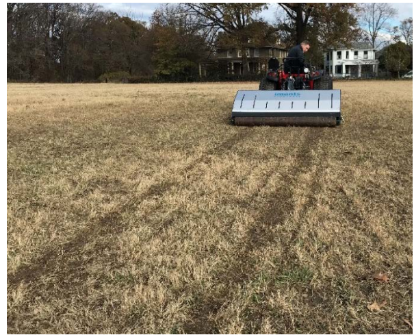
Photo 1 (left): Rotary shaft and blades of rotary de-compactor and Photo 2 (right): tracks left after rotary de-compaction
