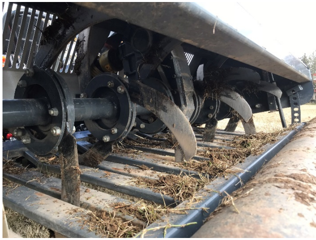
Photo 9: Rotary shaft and blades of rotary de-compactor
