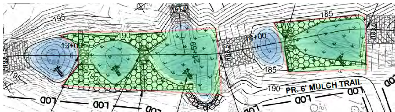
Figure 7: Qualifying floodplain connection area
