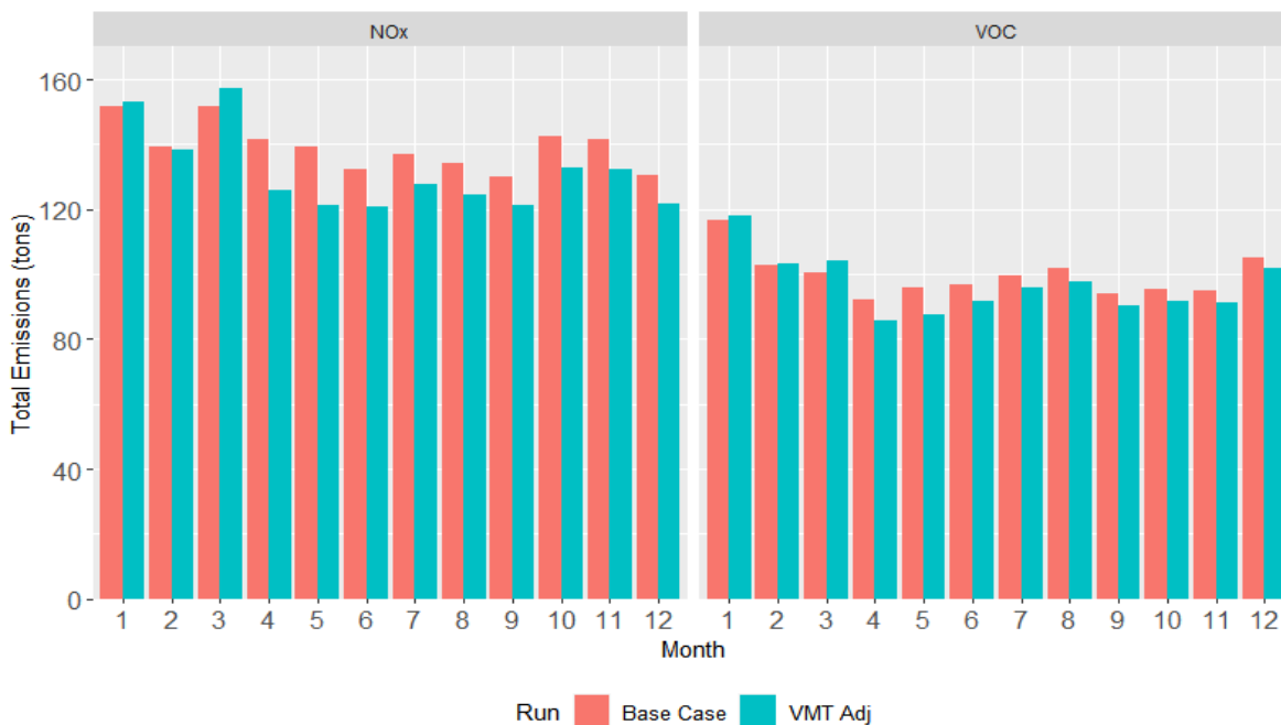
Figure 18: Total NO x and VOCs (tons) from 2019 and 2020 VMT adjusted MOVES run.
