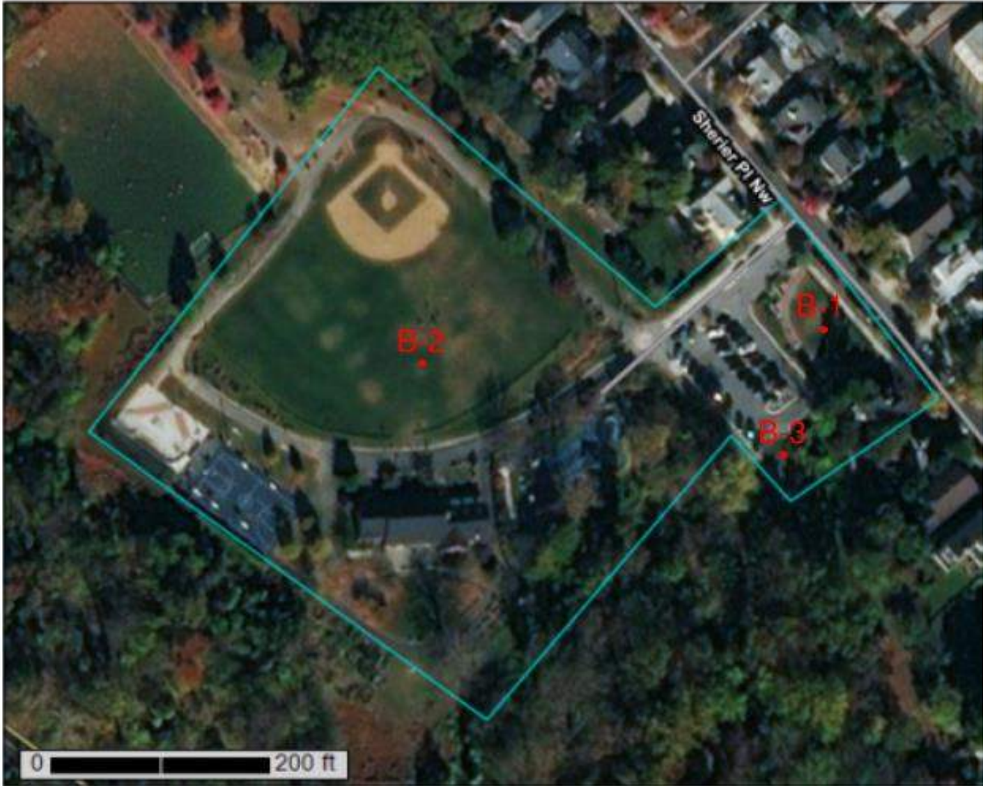
Figure 2 – Soil Boring Locations
