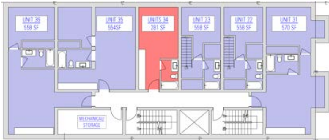
Figure 1: The project's third floor-level includes a variety of floor plans in a modular-friendly configuration constituted of a site-built service core and 7 modules. The westernmost end of the mechanical space affords access to an area where air exhaust and intake is permitted.
